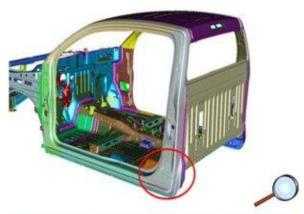
Note: Inspect for the existence of a baffle, positioned between the inner and outer C-pillar sheet metal during the body shop production process. Though not visible from the exterior, its left side location is shown circled above.
