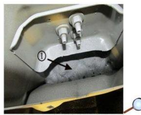
2. Access the open pocket in the inner sheet metal.
